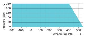
The temperature and pressure recommendations in the graphs apply to gaskets with a thickness of 2.0 mm and smooth flanges. Higher stresses are possible when thinner gaskets are used.
