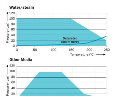
The temperature and pressure recommendations in the graphs apply to gaskets with a thickness of 2.0 mm and smooth flanges. Higher stresses are possible when thinner gaskets are used. Example for the most commonly used other media. Exact data for specific, individual cases are available on demand.
