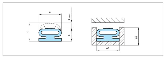
Figure 13 Low-Pressure – with peaked sealing profile
