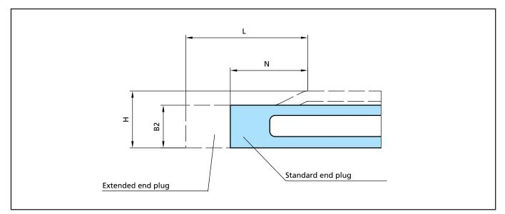
Figure 37 End plugs for high-pressure profile
