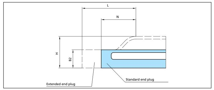
Figure 39 End plugs for low-pressure profile
