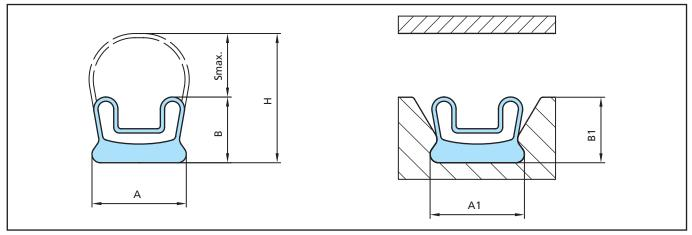
Figure 21 Low-Pressure – smooth sealing surface
