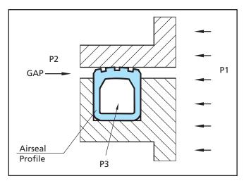
Figure 2 Pressure on Airseal
