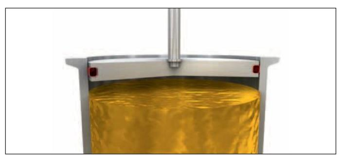
Figure 28 The Airseal expands radially outward against the inside of the drum, sealing the required gap and providing leak-tight operation under pressure.
