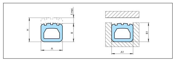
Figure 24 High-Pressure – with smooth sealing profile and grooves
