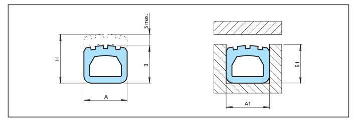
Figure 25 High-Pressure – with smooth sealing profile and grooves
