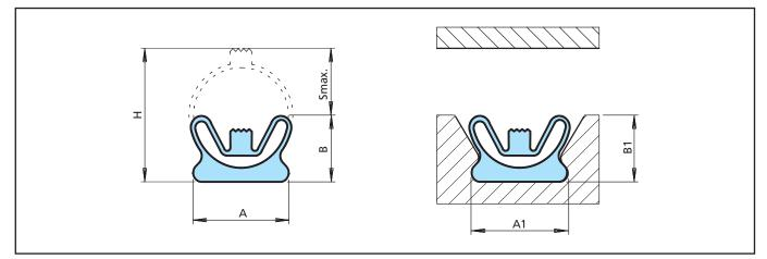
Figure 19 Low-Pressure – particularly pronounced sealing edge
