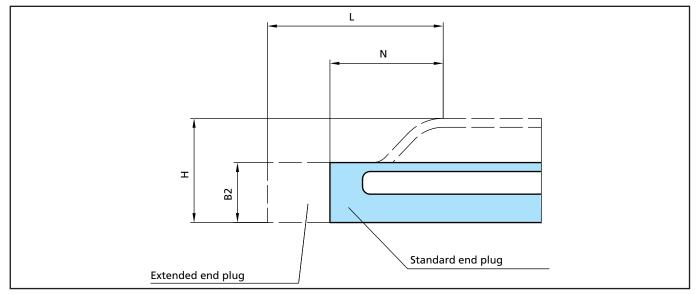
Figure 40 End plugs for low-pressure profile
