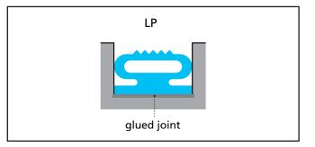
Figure 6 Installed low-pressure Airseal in groove
