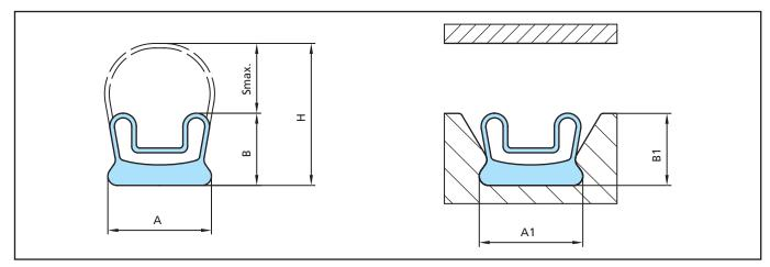
Figure 20 Low-Pressure – smooth sealing surface
