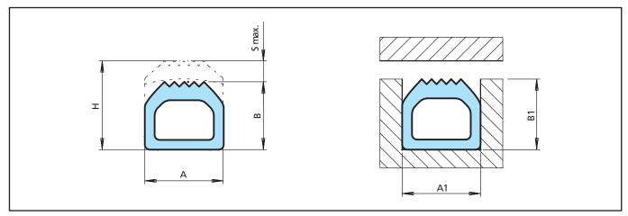
Figure 26 High-Pressure – with peaked sealing profile
