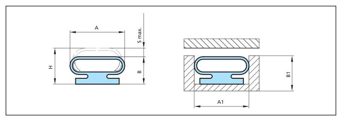
Figure 17 Low-Pressure – with smooth wide sealing surface
