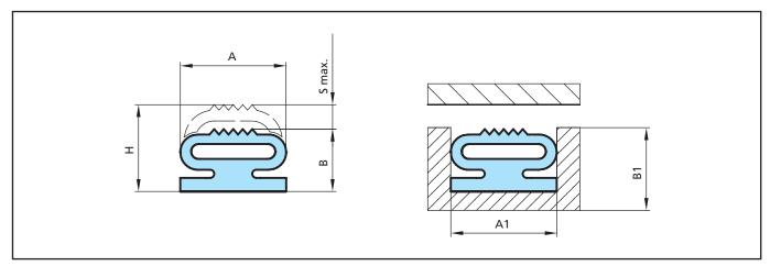
Figure 12 Low-Pressure – with peaked sealing profile
