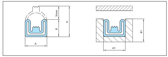
Figure 23 Low-Pressure – with specially formed sealing edge
