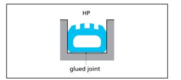
Figure 5 Installed high-pressure Airseal in groove
