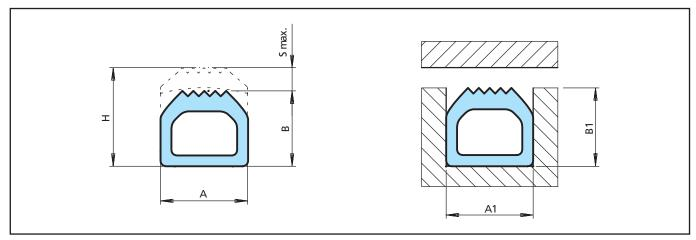
Figure 27 High-Pressure – with peaked sealing profile
