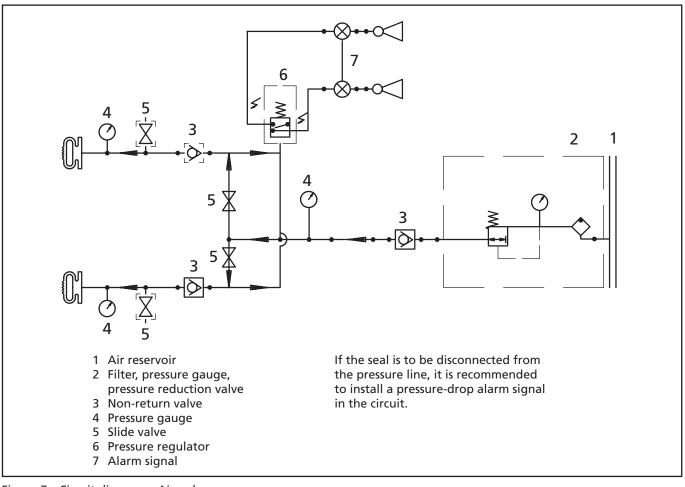
Figure 7 Circuit diagram – Airseal
