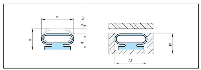
Figure 15 Low-Pressure - with smooth wide sealing surface
