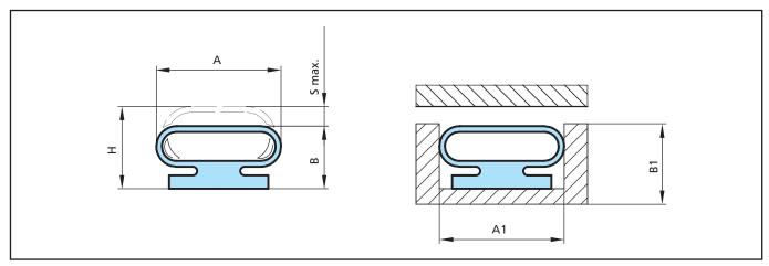
Figure 16 Low-Pressure – with smooth wide sealing surface
