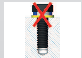
No locking function when combined with flat washers
