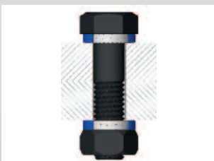
Hexagon bolt in a through-hole, secured on both sides
