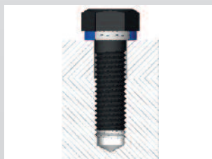
Hexagon bolt secured in a blind hole
