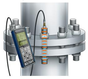
The echometer units work with all bolt tightening systems and are used to monitor the fastener during the tightening process to ensure accurate initial loading. The retained load in the fastener can then be monitored at any time.
